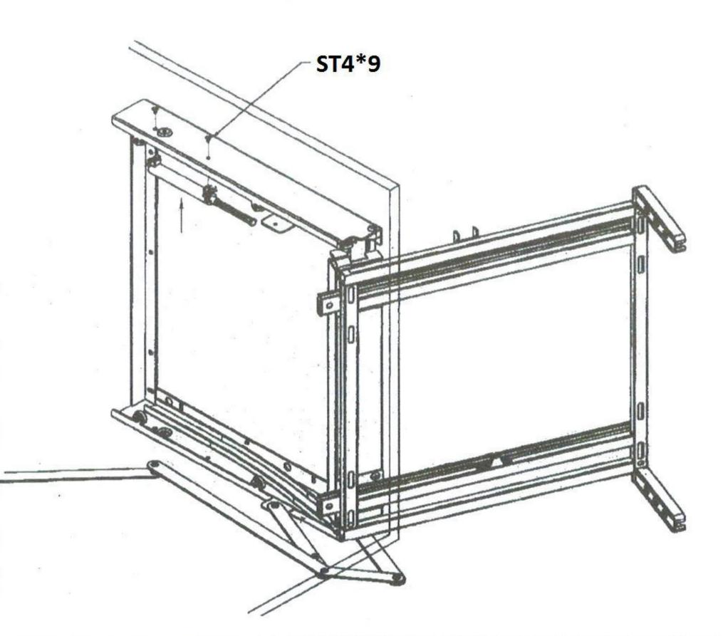
Complete the installation and commissioning, tighten all screws. (Note: this products can be installed left or right, pay attention to adjust the mounting direction of the connecting rod).
