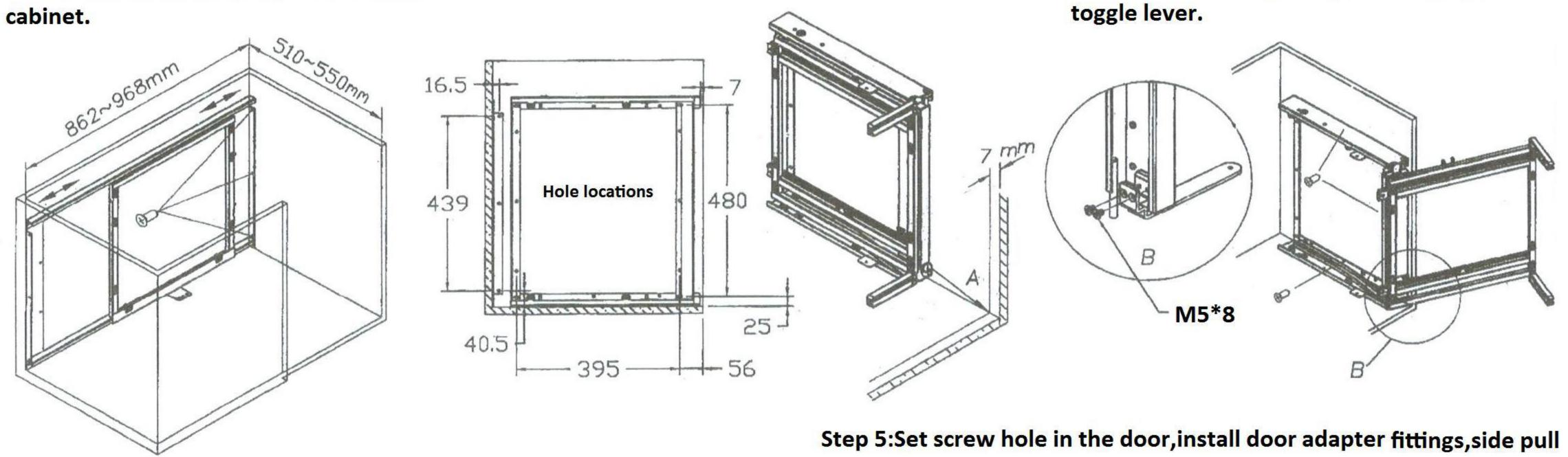
Step 4:Through the connecting rod(as shown), connect the side frame and rear frame connecting slide, and install the door adapter to the side pull frame.
